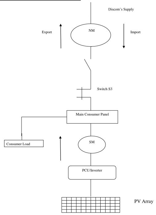
Normally, Solar Generation shall be connected with Grid. When grid fails, Inverter controlled Switch S3 Opens and on restoration of grid S3 Closes.
